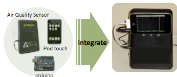
Figure 2. Components of the system (left) and the integrated system, inAir (right)
